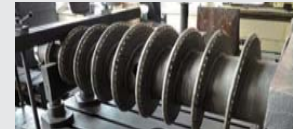
Conveyors Edge Coated With hard surface alloy
