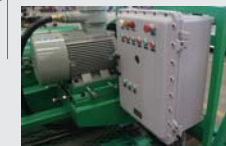
Motors Can Be Atex Certified. Control Cabinet Can Be Atex Certificated(Aluminum Alloy)
